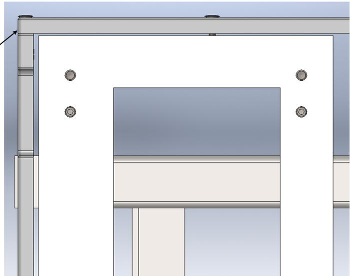
3. Once the panels are attached to each other (effectively creating a box around the bath), the complete inner panel assembly can be secured to the main framework using 4 M6 x 40 countersunk bolts (2 per side panel), which screw into the threaded holes on the bottom frame of the bath. As before, these are finished off with a white cap which pushes into the hexagon socket of the screw. **There should be a gap of approximately 3mm between the bottom of the end panels and the floor.**
