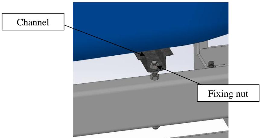
There are 6 grub screws, each located next to one of the fixing points, which can be used to allow for any slight deviations in the floor surface, and also to ensure that the bath is perfectly level. Ideally the frame will be fixed tightly to the surface of the floor, and the grub screws will not be
